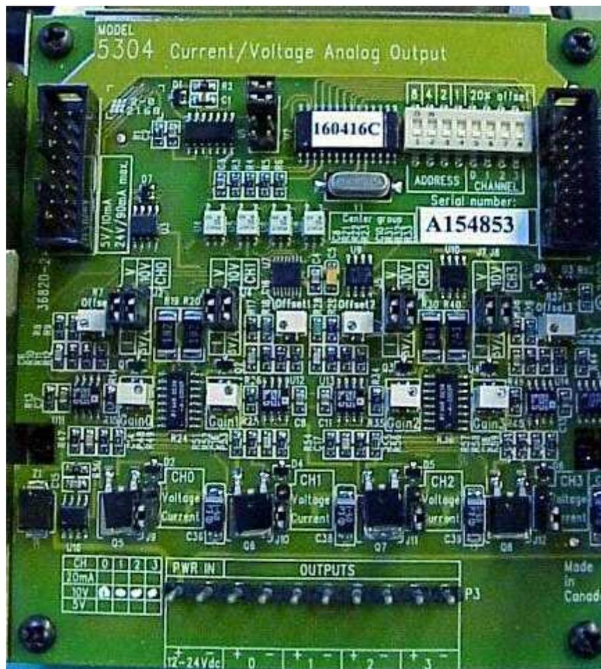
**Figure 6: Location of Gain and Offset potentiometers.**
